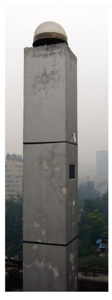
The fiducial station on the Sichuan seismic and active control network. This was a "sunny" day; pollution has taken its toll (that used to be a clear dome!).
